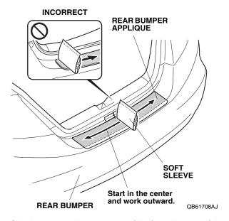
Slowly remove the protective film from the top of the rear bumper applique. Remove the protective film by pulling it slowly and horizontally; do not pull it vertically.
